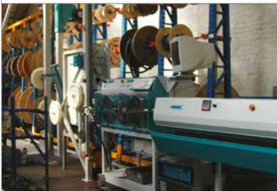
AUTOMATIC CABLE CUTTING & PREPARATION
